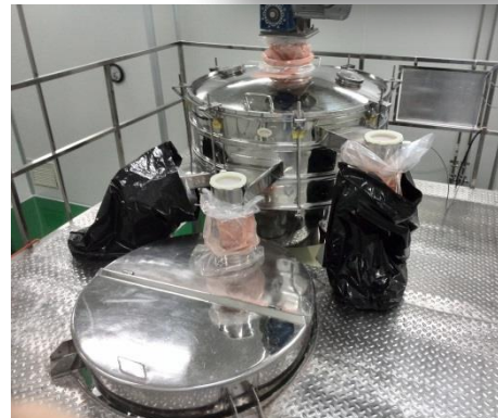
A 1200 mm Tumbler Screen double-deck with a 40# & 80# screen, Processing 2t/h capacity of pharma powder
