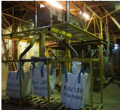
A Rotary Sifter- W1000xL3000mm double deck for grading lime sand at size 30/35/42#, Capacity 10t/hr
