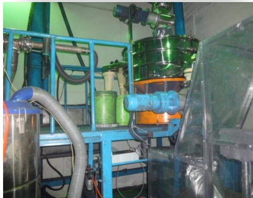
A 1000 mm Vibrating Screener single-deck with a 400# screen, Processing 400kg/h output lithium cobalt oxide
