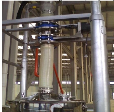
A 600 mm Vibrating Screener with a 100# screen, Processing 500kg/h capacity food additives
