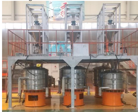
Ultrasonic Vibrating Screeners for processing Titanium oxidized 400/500# with airlock feature
