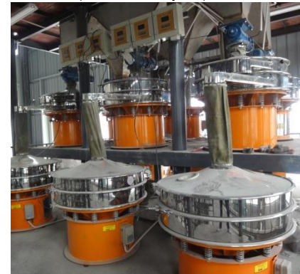
89 sets of Ultrasonic Screener for sieving 600# Silicon at 3000t/month productivity, which meet JIS standard required d50 volume ranging from 18.5-21.5
