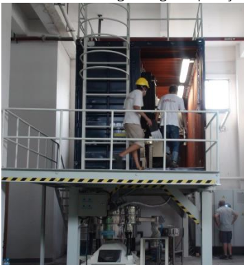
A 1200mm Tumbler Screen for sifting plastic with nitrogen introducing
