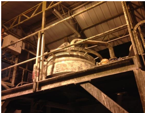
A 1200 mm Flow Thru Screener with a 18 # screen, Processing 20t/h capacity of hydrated lime
