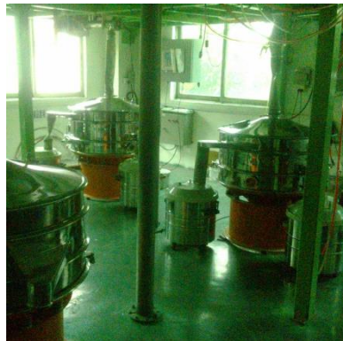
1000mm Vibrating Screeners (5sets) for grading solder powder at size 325# & 400#
