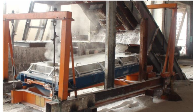
Dimension W1500xL3000mm Gyratory Screener double-layer with a 40# and 55# screen, Processing 5t/h capacity sodium carbonate
