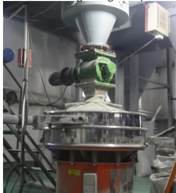
A 1000 mm Vibrating Screener with a 320# screen, Processing 2t/h capacity of adhesive
