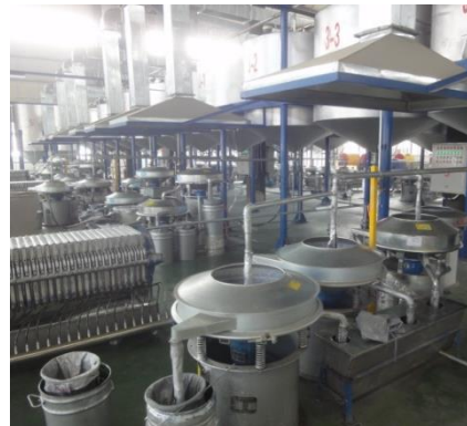
80 sets of High Frequency Filter for purify aluminum past of 5000t/year production
