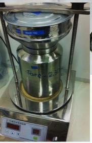
A tailor madeNV300 Tester for analyzing high end ceramic powder collected as Zirconium Oxide-stabilized Substrates for quality assurance.
